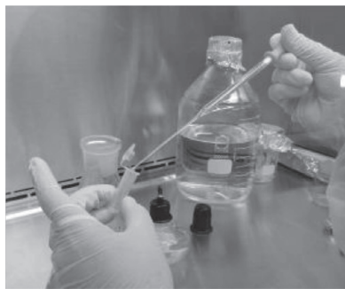
Removing a culture aliquot for reading under a microscope
